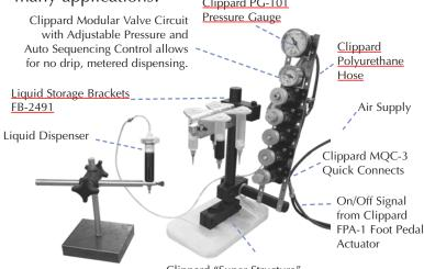
Clippard "Super Structure" Squeeze Block Adjustable Fixturing
